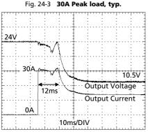
High Overload Current (typ. 30A for 12ms) enables easy fuse tripping
