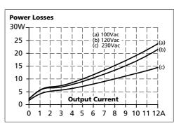
Fig. 9-4 Losses vs. input voltage at 24V, 10A,
