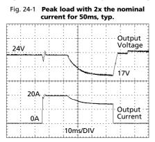
20A Peak load (resistive) for 50ms Output voltage dips from 24V to 17V.
