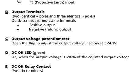
Monitors the output voltage of the running power supply.
