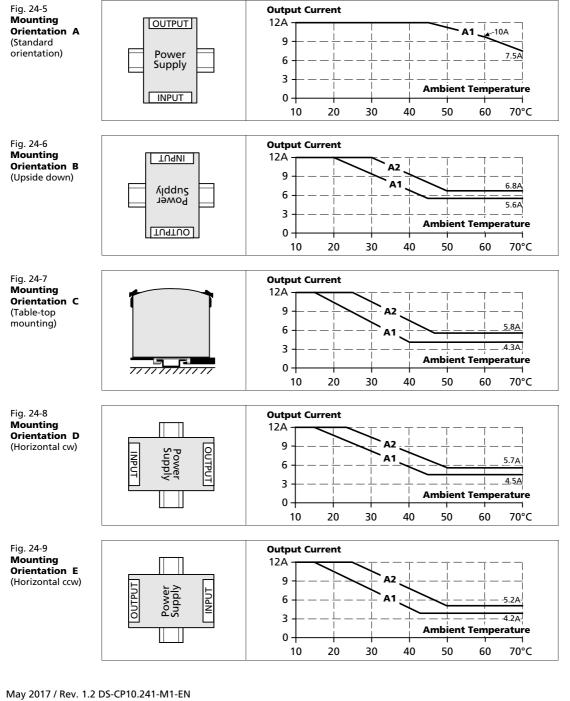
All parameters are specified at 24V, 10A, 230Vac, 50Hz, 25°C ambient and after a 5 minutes run-in time unless otherwise noted.
