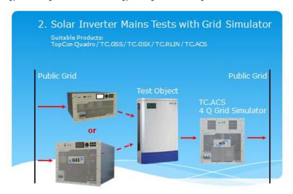
All relevant test procedures according to IEEE- and VDE- can be performed, the high degree of programmability gives room for any kind of later extensions. As all REGATRON power supplies, TC.ACS units may be paralleled in order to have full bidirectional power systems up to the MW-range.
