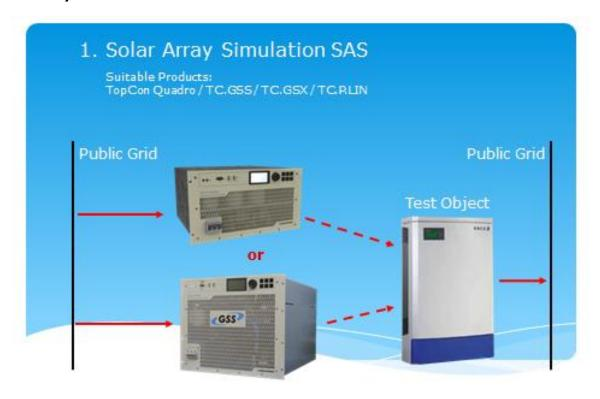
**TopCon Quadro as also bidirectional TC.GSS** power supplies provide full Solar Array Simulation capability alongside with all relevant DC applications. Note especially, that on the contrary to the most competitors REGATRON DC power supplies are processing relevant SAS data in real-time on-board of the power supply.
