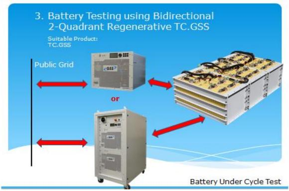
Regenerated energy is reinjected into the public grid with a very high efficiency and a perfect power factor.
