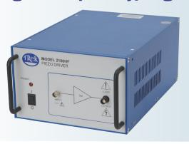
The Trek Model 2100 HF is a high-frequency, high-speed, wide bandwidth amplifier for high power applications. It incorporates an all-solid-state design for highly reliable low-noise operation, thus achieving accurate output response and high slew rates, even in highly capacitive loads. Full power frequency response of the amplifier is essentially flat up to 2 MHz. No overshoot or instability of the waveform occurs due to the amplifier's unique dual feedback feature.
