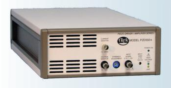
The Trek Model PZD350A is a high-voltage DC-stable piezo driver/amplifier designed to provide precise control of output voltages in bipolar or unipolar ranges that are customer specified within a range of available settings. It is configured as a noninverting amplifier with a variable DC gain. An inverting amplifier configuration is also available.
